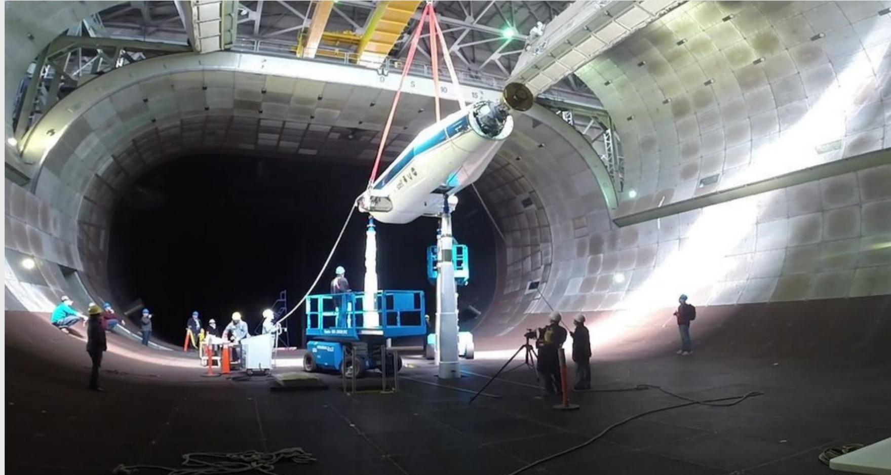
Arnold Engineering Development Complex crew members lower the NASA/Army Tiltrotor Test Rig into the 40-by 80-foot wind tunnel at Moffett Field in California. (Photo credit: U.S. Air Force)
